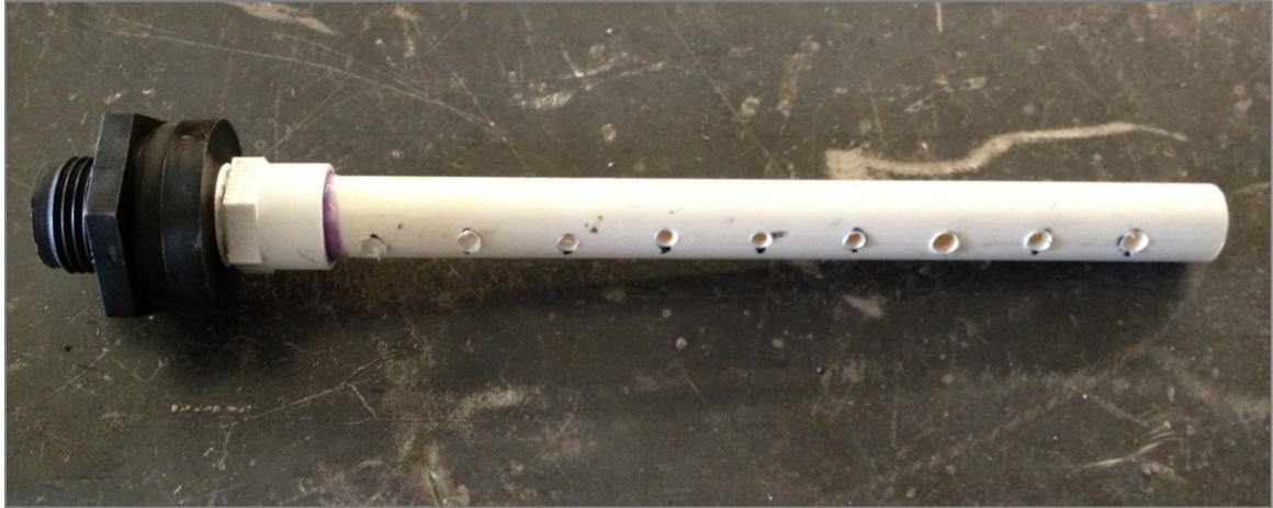
Figure 7: Perforations in the PVC underdrain prior to wrapping with permeable felt
